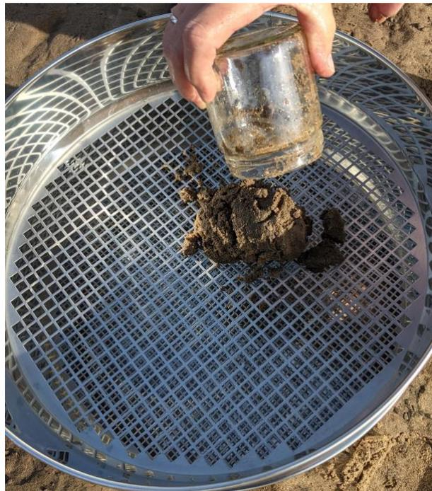
Figure 3: Sediment being emptied into 10mm sieve.
